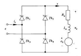
2. A single-phase semiconverter , shown in Fig.2 , is used to control the speed of small separately excited d.c. motor rated at 4.5 kW, 220V, 1500 rpm. The converter is connected to a single – phase 230 V, 50 Hz supply. The armature resistance is Ra = 0.50 ohm and the armature circuit inductance is La = 10 mH. The motor voltage constant is Ke  $\Phi = 0.1$  V/rpm.
