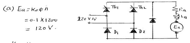
$$V_{a} = V_{dc} = E_{a} + I_{a} R_{a}$$
